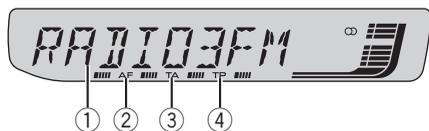
RDS (radio data system) is a system for providing information along with FM broadcasts. This inaudible information provides such features as program service name, program type, traffic announcement standby and automatic tuning, and is intended to aid radio listeners in finding and tuning in to a desired station.
